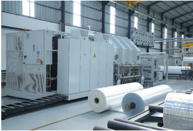
2500 mm Metallizing Machine (Buhler Germany)
