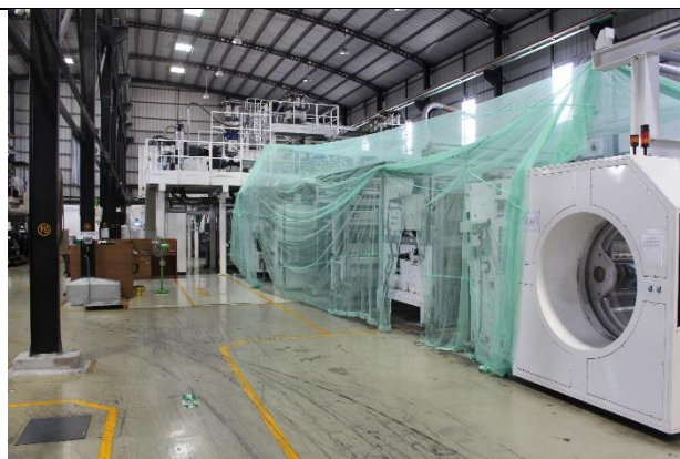
2500mm CPP/CPE Film Manufacturing line with MDO (Colines Italy)
